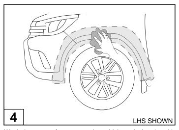
Wash the areas of contact on the vehicle and wipe dry with a clean cloth.
