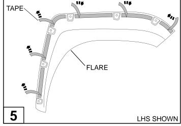
On the inside of the fender flare remove approximately 25mm of the protective liner from all the double sided tape locations. Fold the liner over and secure with masking tape to the outside of the fender flare.
