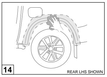
Wash the areas of contact on the tub as shown and wipe dry with a clean cloth.
