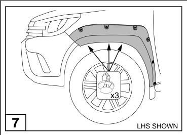
While pressing and holding the fender flare in position of best fit, secure the fender flare with 3 plastic scrivets previously removed in step1.
