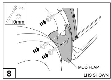
Using 10mm spanner or Phillips head screwdriver secure the mud flap and fender flare using 3 new screws supplied.
