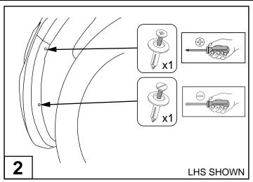
Using Phillips head screwdriver remove and discard the top scrivet from the front bumper bar inner arch. Using flat screwdriver remove and discard the lower plastic scrivet as shown.
