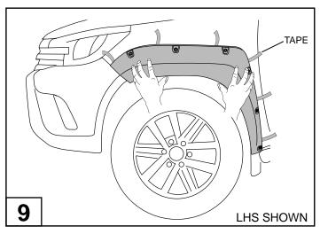
Once the fender flare is fitted, pull all exposed liners at right angle to flares. Apply pressure around edge of the fender flare to achieve proper adhesion.
