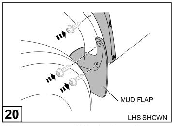
Using 10mm spanner or Phillips head screwdriver secure the mud flap and fender flare using 3 new screws supplied.
