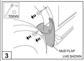
Remove and discard the 2 screws holding mud flap and 1 screw from the wheel arch as shown. Use 10mm spanner or Phillips head screwdriver. Mud flap will still remain attached to the vehicle.
