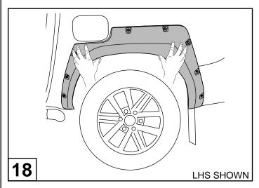
Fit the fender flare to the vehicle as shown.
