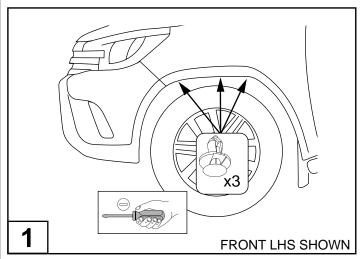
Using flat head screwdriver remove and retain the 3 plastic scrivets from the front fender as shown.
