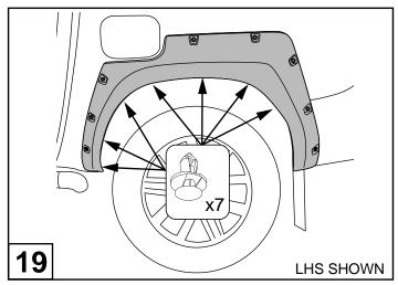
While pressing and holding the flare in position of best fit, secure the fender flare with 7 plastic scrivets previously removed in step15.
