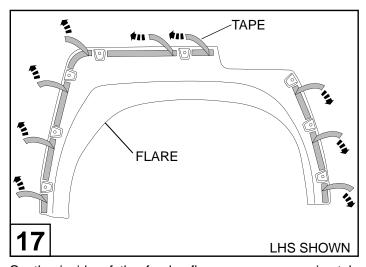
On the inside of the fender flare remove approximately 25mm of the protective liner from the double sided tape locations. Fold the liner over and secure with masking tape to the outside of the fender flare.
