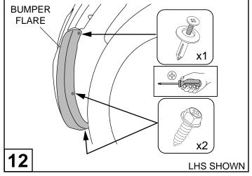
Using 10mm spanner or Phillips head screwdriver secure the bumper flare with 1 new screvet and 2 new screws supplied, as shown.
