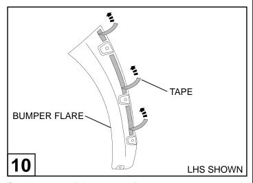
On the inside of the bumper flare remove approximately 25mm of the protective liner from the double sided tape locations. Fold the liner over and secure with masking tape to the outside of the bumper flare.
