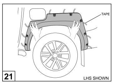
Once the fender flare is fitted, pull exposed liners at right angles to flare. Apply pressure around edge of fender flare to achieve proper adhesion.
