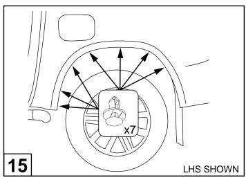
Using flat head screwdriver remove and retain the 7 plastic scrivets from the rear fender as shown.
