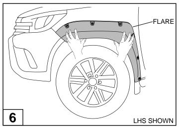
Fit the fender flare to the vehicle as shown.
