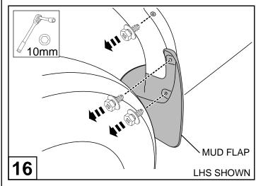
Remove and discard the 2 screws holding mud flap and 1 screw from the wheel arch as shown. Use 10mm spanner or Phillips head screwdriver. Mud flap will still remain attached to the vehicle.
